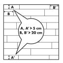
Before starting, carefully measure the length and the width of the room to plan a precise layout to achieve a balanced appearance of the floor. As shown in the image, A and A' not less than 5 cm & B and B' more than 20 cm.
