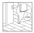
If the doorframe is installed after the floor installation, please make sure that a min. 1mm vertical gap is left between the base of the doorframe and the surface of the floor.
