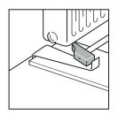
In places where it is difficult to install the planks with the tapping block (e.g. underneath radiators), you can tap them together with the pulling iron and a hammer.
